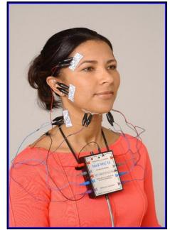
Fig 2: Electromyographic sensors attached to the face[11]
