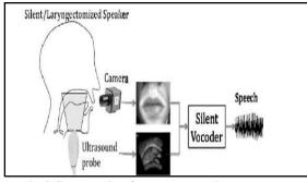
Fig 3 Schematic of ultrasound silent sound interface[13]
